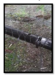
All fence posts and debris can be rolled up with the mesh, all loose wire and barbed wire is simply moved into the centre of the mesh and wound up with the ring-lock decreasing the time to remove the old fence and effecting a neat and tidy package for recycling
